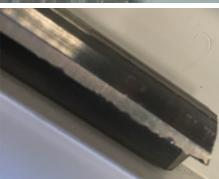
This results in chipped teeth on the saw blade that cannot be repaired or re-sharpened, and if undetected will lead to **chipped profiles**, accuracy problems and will **permanently destroy** the saw blade.
