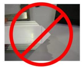
Do **NOT** check the arrow head position with a square across the small face. This has been known on several occasions to show an error on the profile, and fools the unwary into an adjustment of the central position. This happens because the narrow part of the profile has not been extruded square to the bottom face.
