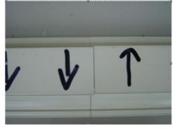
This picture shows a poor quality profile where the narrow face is not centralised to the rest of the profile. The outer edges are lined up, but it is clear that the narrow edges are not.
