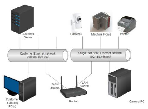
The new Router forms a bridge between the customer's network and ours. This means the IP range on the customer side can be anything, yet on the Stuga side, the network range and IP addresses can be fixed tin the range 192.168.116.1 to 192.168.116.255.
