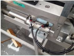
Sensor P0001013 should be labelled X001 and has cable and M8 connector already attached. Plug into FB06A port 2. Reed switch needs P0001041 mounting bracket and P0001042 mounting band to fix to cylinder body.
