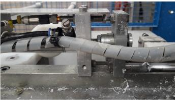
Step 2 - Ensure the profile bottoms out on the gripper nose not holder
