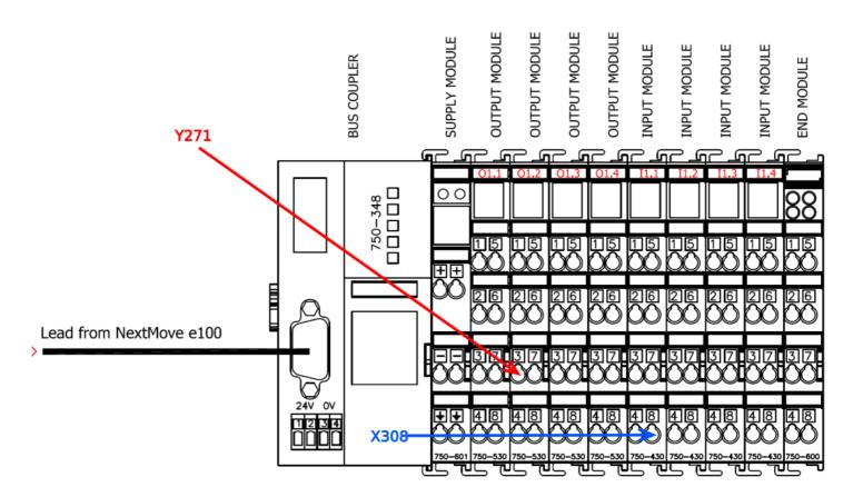
• New Cable X308 (InA\_InvZero) from M2, connect to input channel 8 on 1st IO slice (labelled 8).
