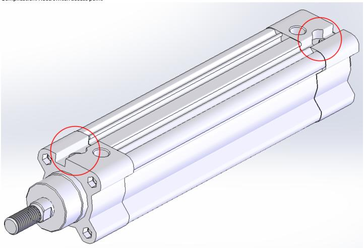
The original Festo cylinders fitted to Microlines and ZXs had an access point for the reed switch. This allowed Festo reed switches of type 150855 to slide in. This type of Festo reed switch has been replaced by a version (SME-8M) that does not need to slide in - it drops in and locks off. This type of cylinder is no longer available which leaves a Reed switch compatibility problem
