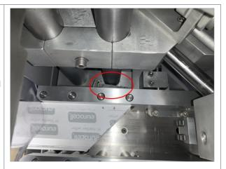
The saw infeed is stopping the profile being correctly positioned on the rear fences.
