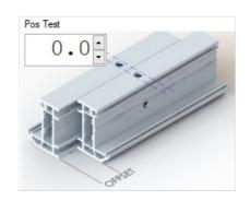
...The machine tolerance is +/0.5mm, so there is no need to adjust if an inaccuracy is less than this tolerance (1mm back to back)
