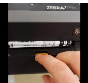
On Zebra ZD620, ZD420, ZD421 printers in peel-off mode, the labels do not peel off cleanly and bunch up on the reel
