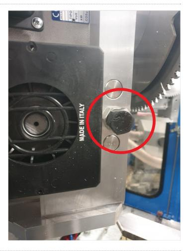
Step 3 - Slacken off four bolts on adjusment mechanism.
