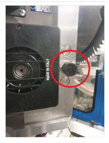
Step 3 - Slacken off four bolts on adjustment mechanism.
