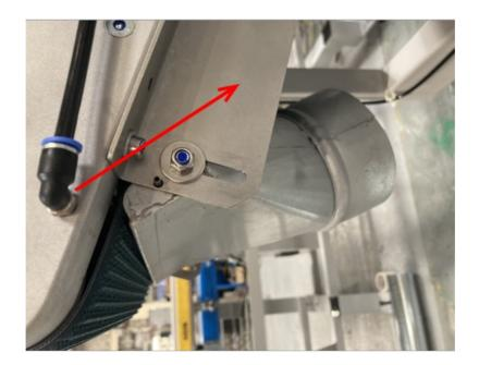
ensure gap is less than 5mm between nozzle and belt then fit a 3 mm roll pin drilled through both parts to stop bolts acting as a pivot
