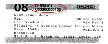
The first number circled is the batch number, and the second is the piece number within that batch. The labels produced on your machine may be slightly different depending on setup.
