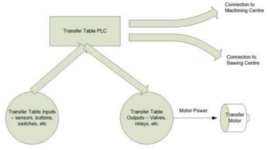
The transfer table control comes from a PLC in the transfer table cabinet. It communicates with the Machining centre in that it tells the software if the first sensor position is free (Ready To Accept)
