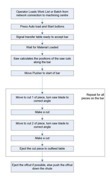
A batch is loaded into the saw across a network connection. The operator presses auto load and start and the next bar is loaded from the transfer table. Each cut piece consists of two cuts – lead and tail. The pusher pushes the profile to the position for the lead cut, the saw head rotates to the correct position. The cut is made. The same process is repeated for the tail cut, but as the piece is cut through, the piece is ejected onto the outfeed table.
