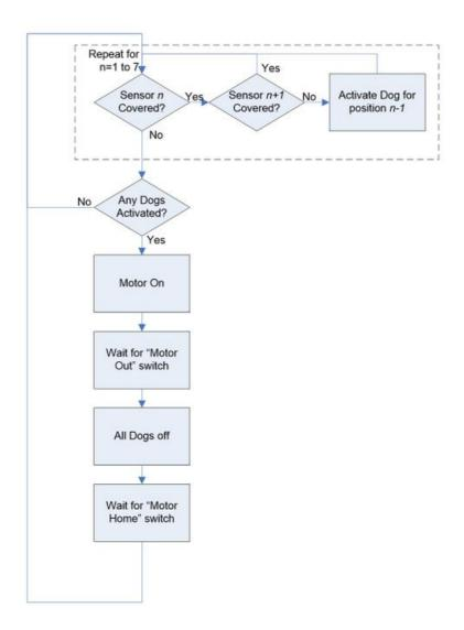
The sensors on each station detect if a bar is there. If a bar exists and the neighboring space is empty then activate the dog. This is repeated for each station. If any dogs are activated, then run the sequence to move the bars along one station.
