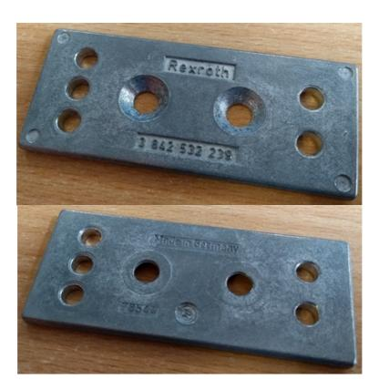
Simply countersink the centre of the 3 holes shown on the left hand side. The countersink should be done from the face shown, and should allow for an M5 countersunk screw to fit flush or subflush, but without the countersink section of the screw breaking through the far face of the plate.
