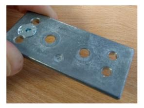
When fitting, the top hat can then slide fit over the screw as normal (note: it will be a looser fit than with the dowel, but will be captivated when the door is installed).
