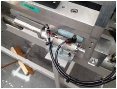
Sensor P0001013 should be labelled X001 and has cable and M8 connector already attached. Plug into FB06A port 2.
