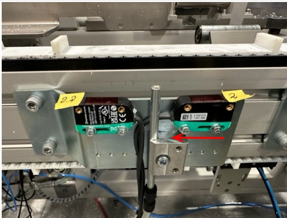
Position of sensors can be adjusted on hole pitch - For 50mm slim outer, the rearmost sensor needs to move forward one pitch
