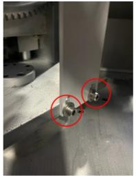
And strengthen the top half moon plate mounting by drilling extra countersunk holes and using M8 instead of M6 bolts It is also possible to utilise the handing hole for an additional screw
