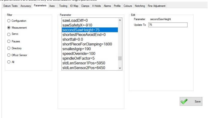
This is the actual height that the user sets the saw blade to lift to
