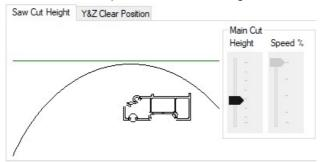
Th physical height of the sensor on the cylinder will need to be adjusted by trial and error to ensure it switches at a similar point to the expectation of the green line
