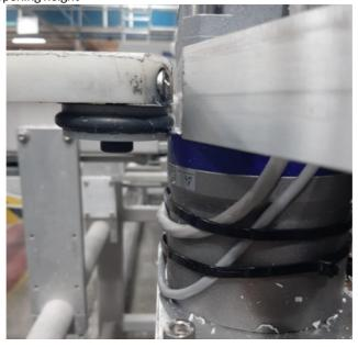
This was overcome by reducing the geabox plate mount width to drop the entire gearbox body blow the zip gates
