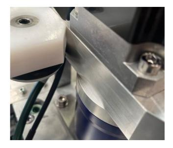
The addition of the rear stainless gate opener allows the opening dimension to be correct and overcome this issue
