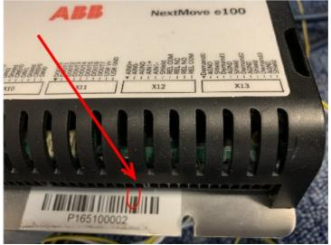
Photo shows the E100 with no connection plugs in A wire link should be inserted between the REL NO and REL COM connections on the X12 connector This has the effect of linking out the Drive Enable relay so it is permanently on
