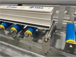
Parts are supplied in R0019181 Kit: Additional Friction Rollers for Toothed Gripper Mk3
