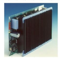
The advanced design of the DM series drive using MOSFET technology enables continuous winding currents of up to 16.5A (peak). In Addition the DM series drives will protect themselves against all motor winding faults including winding shorts as well as supply related faults. For ease of installation we recommend the use of SmartDrive's range of dedicated drive backplanes, for more information contact the SmartDrive Sales department.
