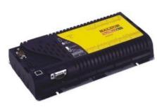
Motion Control, Inputs and outputs are controlled via a Baldor / ABB Nextmove ESB card. This is a programmable device that handles the sequencing of the machine and drives the pusher arm to the correct positions.
