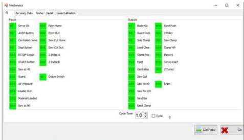
Inputs are the feedback from sensors, buttons and switches and have a code beginning with "X". The state of an input is displayed as:
